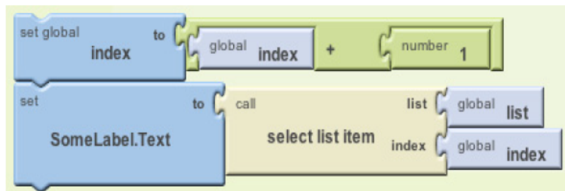
Figure 19-7. Incrementing the index value and using the incremented value to select the next list item
