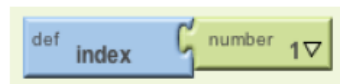
Figure 19-9. Using the index variable, which is initialized to 1, to track the current position in a list
