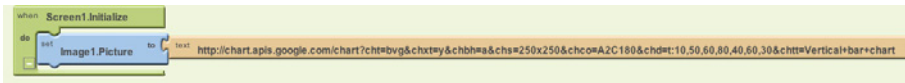
Figure 24-5. When the app starts, it sets the picture to a chart returned from the Chart API URL
