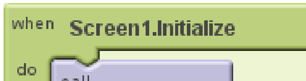
Figure 14-8. Using a Screen1.Initialize event block to move the mole when the app begins
