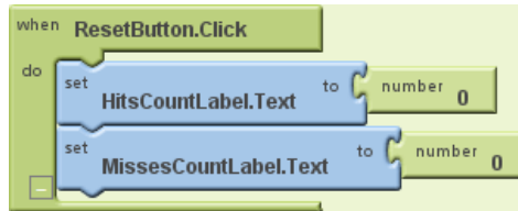
Figure 3-9. Resetting the number of hits ( HitsCountLabel ) and Misses ( MissesCountLabel ) when the Reset button is pressed
