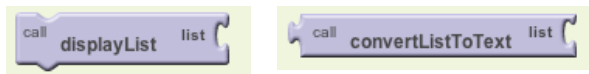
Figure 21-14. The call on the right returns a value and so must be plugged into something
