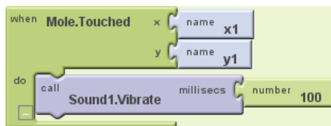
Figure 3-10. Making the phone vibrate briefly (for 100 milliseconds) when the mole is touched
