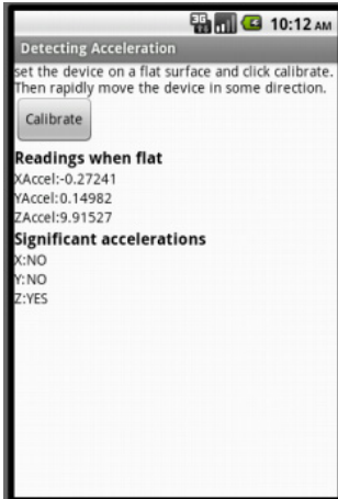
Figure 23-15. Calibrating the acceleration readings
