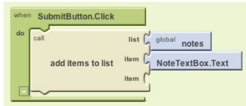
Figure 19-16. Calling add items to list to add the new note when the user clicks the SubmitButton
